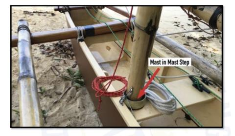
Clip the end of the mast strut to the pre-rigged loops on the piece of bamboo lashed to the cross arms. See photo below:
